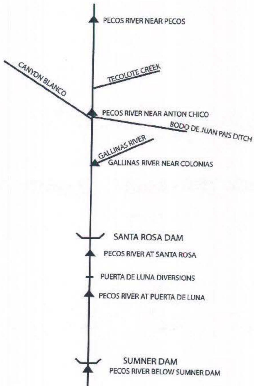
Figure 2 Diagram of Pecos River Near Pecos to Sumner Dam
