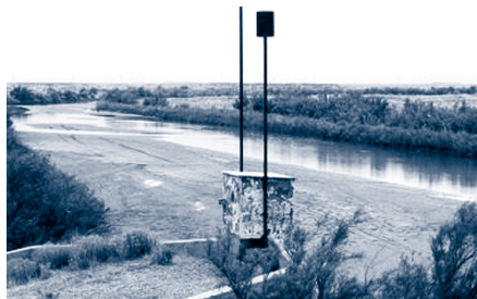
This picture shows how the river sometimes wanders away from the measurement gage.
