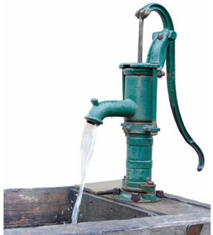
Figure 10-8: A hand pump is an old-fashioned device that requires no electricity to operate—just human muscle power.
