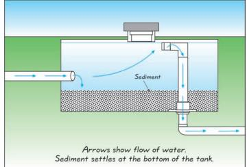
Figure 8-10: Example of a sediment trap. The top photo shows the installation of two traps; the illustration depicts how water flows through a trap.
