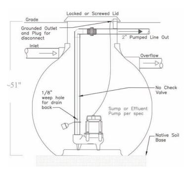
Figure 9-8: A pump tank can be used to pump water into a system's main water storage tank.
